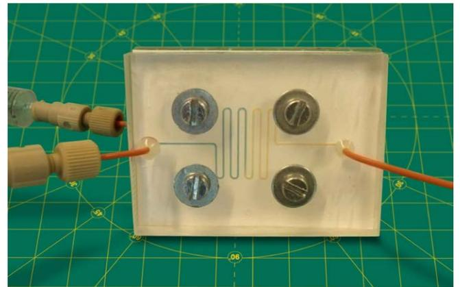
Micro reactor used for testing the CO<sub>2</sub>-permeability of membranes (source: University of Twente, NL)
