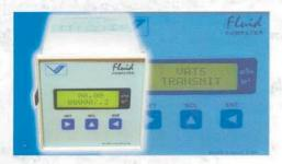
Description: VATS J-510 Flow transmitter converts the flow-sensor [JT-121] signal into the required engineering units with the help of Microprocessor based electronic module to indicate flow rate, total flow or control a batch or to run a PID controller. 4-20 mA current output is a standard feature. Computer compatibility with RS-232 or RS-485 interface is an add-on feature as optional.
